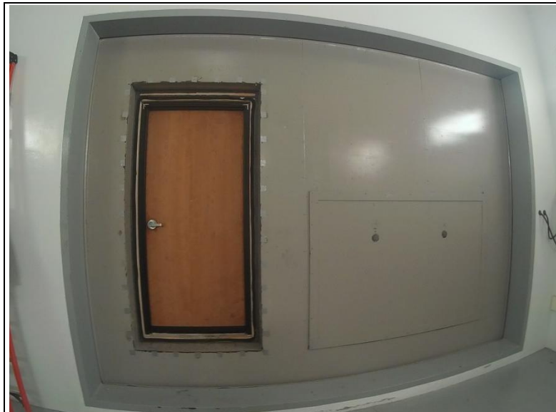
Photo No. 1 Source Room View of Installed Specimen
