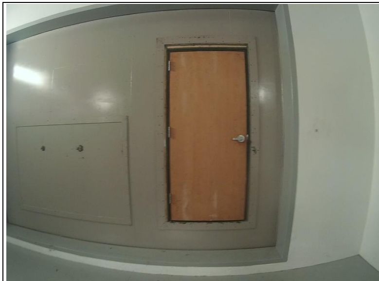
Photo No. 2 Receive Room View of Installed Specimen
